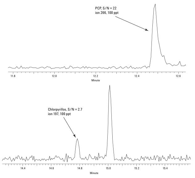
Figure 3. Extracted ions for PCP and chlorpyrifos.
