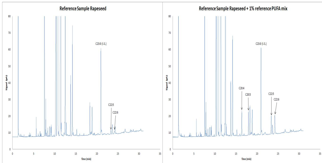
Figure 4: Reference biodiesel sample (rapeseed source). Sample contains < 0.1 % PUFA methyl ester.
