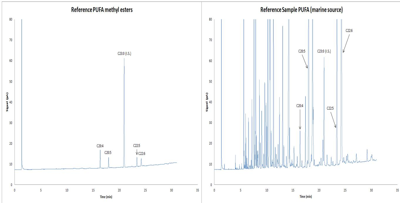
Figure 2: Chromatogram of Reference sample, containing the four predominant PUFA methyl esters and Internal standard (C<sub>23:0</sub>)
