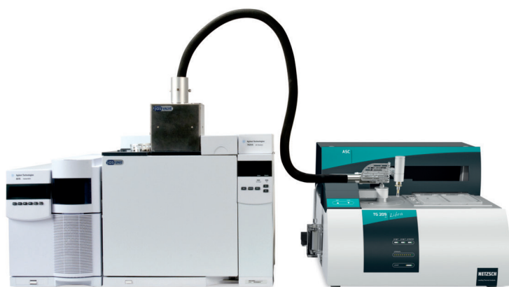
2 NETZSCH TG 209 F1 Libra ® TGA instrument coupled to the Agilent 7890A gas chromatograph equipped with an Agilent 5975C quadrupole mass spectrometer (QMS)
