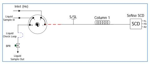
Figure 1: Plumbing diagram for Sulfur Compounds in Light Petroleum Liquids analyzer according ASTM D5623 using PAC SeNse detector (with optional LSV)
