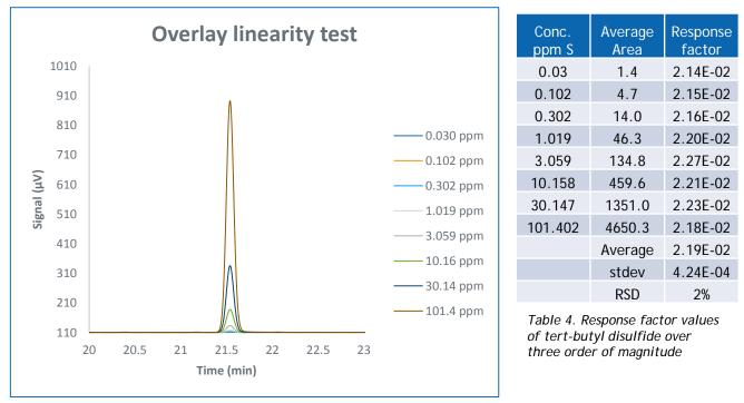
Figure 6: Linearity overlay of 30 ppb to 100 ppm tert-Butyl Disulfide
