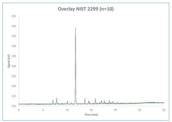
Figure 5: Repeatability overlay of 10 consecutive runs of NIST 2299 in ASTM D5623 ALS injection.
