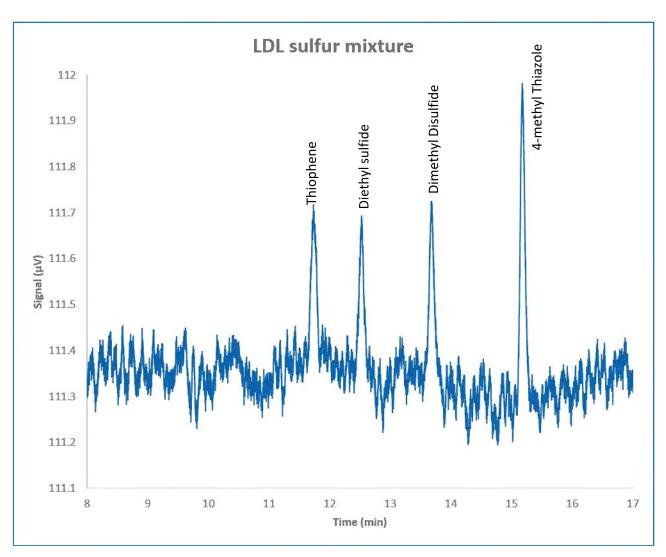
Figure 8: Chromatogram of SeNse check mix diluted to ~ 40 ppb / 100 ppb
