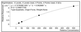
Figure 3: Calibration for Napthalene (25 to 500 µg/L)
