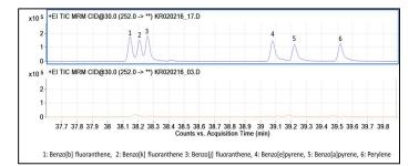
Figure 5: LOD standard @ $2.5\mu$ g/L (top trace in blue) and matrix blank (bottom trace) following SBSE clean up (MRM 252>)
