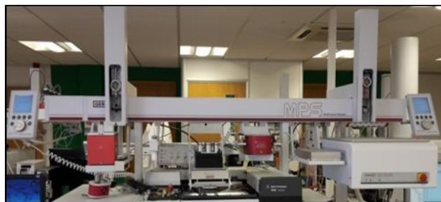
Figure 1: GERSTEL Dual Head MPS for fully automated direct fatty acids trans-methylation
