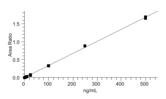
Figure 5. Linear calibration function for NMDA from 1 ppb to 500 ppb
