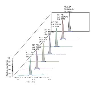
Figure 4. NDMA calibration runs from 1 ppb (bottom) to 500 ppb (top)
