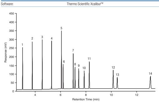
Figure 1: 1% C8–C24 FAMES solution separated on a TraceGOLD TG-WAXMT metal GC column
