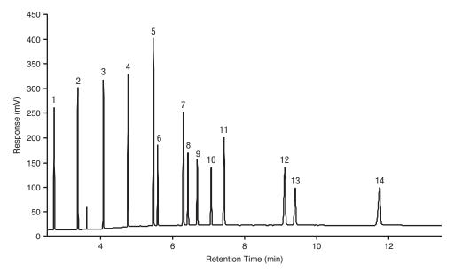
Figure 2: 1% C8–C24 FAMES solution separated on a TraceGOLD TG-WaxMS fused silica GC column
