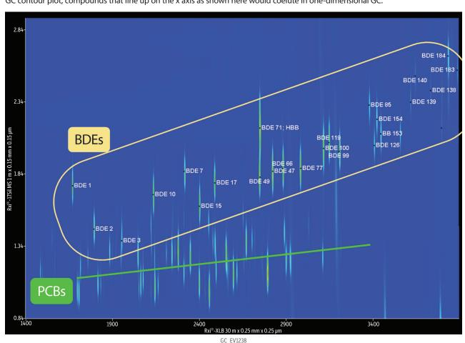
**Figure 5:** PCBs and BDEs are easily determined using GCxGC-ECD with Rxi<sup>®</sup>-XLB and Rxi<sup>®</sup>-17Sil MS columns. In a two-dimensional GC contour plot, compounds that line up on the x axis as shown here would coelute in one-dimensional GC.
