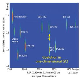
PCBs and BDEs will coelute; however, the second dimension Rxi®-17Sil MS column helps resolve BDEs from PCBs (Figure 9). To learn how we developed our sample preparation technique for this analysis, search for "milk matters" at **blog.restek.com**
