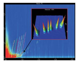
Figure 3. Expanded 3D display of HBDE isomers.
