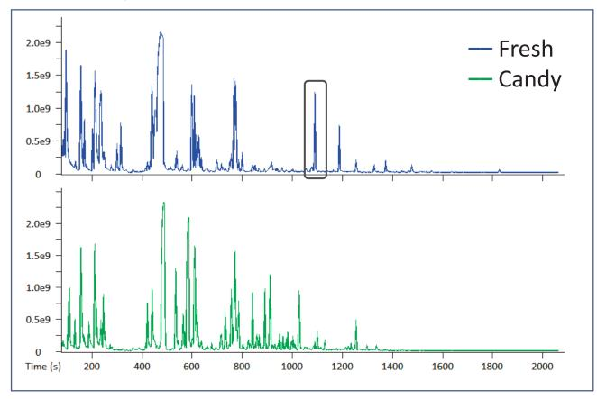
Figure 1. Total ion chromatograms (TICs) for a strawberry-flavored candy and a fresh strawberry are shown. These samples have dramatic differences with hundreds of analytes observed in each.
