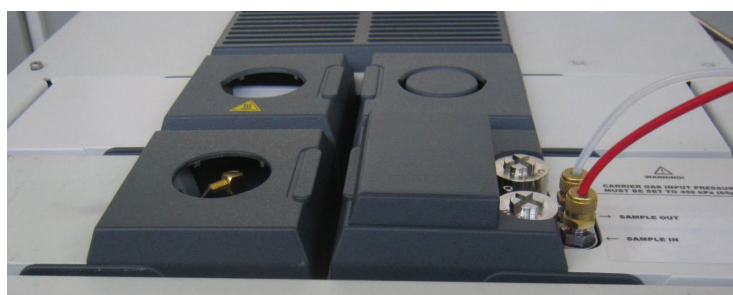
FIGURE 2. TRACE 1300 GC equipped with GSV module and FID-TCD in series.
