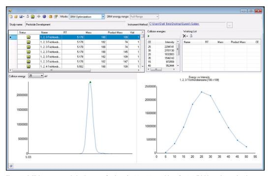
Figure 2. Collision energy optimization curve for the m/z 180 > 109 transition of 1, 2, 3-Trichloroethane, showing an optimum collision energy of 25 eV. At this point in the process, the optimized SRM transitions can be exported to your instrument method.
