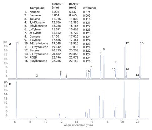
**Figure 4.** Without using RTL, chromatograms of 15 compounds analyzed by the ASTM D7504 method, front and back.
