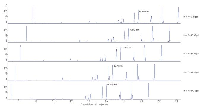
Figure 2. RTL calibration runs using o-xylene as the RTL target peak.
