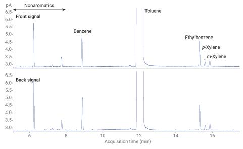
Figure 7. Toluene solvent with RTL.
