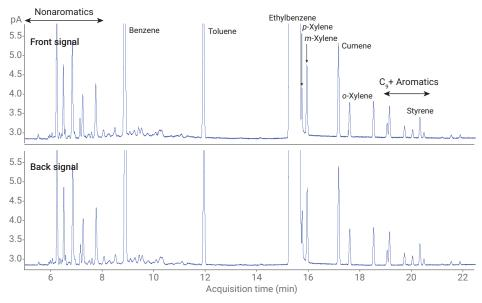
Figure 8. Ethylbenzene solvent with RTL.
