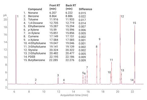
Figure 5. Using RTL, overlay of 15 compounds analyzed by the ASTM D7504 method, front and back.
