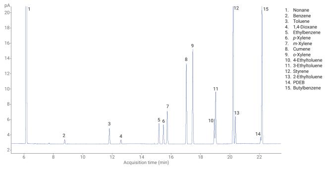
Figure 1. Chromatogram of the 15 compounds analyzed by the ASTM D7504 method.
