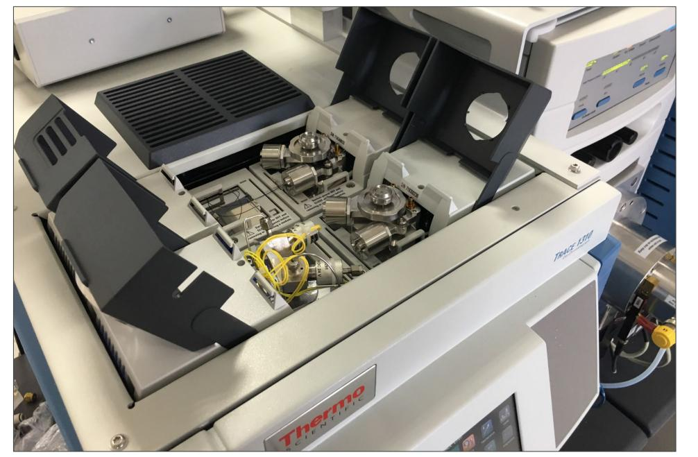
Figure 4. TRACE 1310 GC with DualData XL module (left front slot), standard SSL Injector (right front slot) and the Instant Connect Helium Saver Injector Module (back slots) mounted on the DFS Magnetic Sector GC-HRMS.
