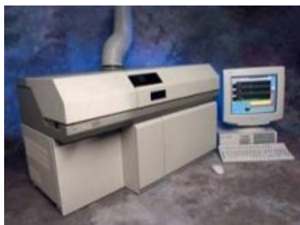
Figure 2. The HP 4500 was the world's first computer controlled benchtop ICP-MS, introduced in 1994.
