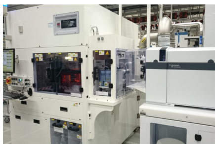
Figure 9. A fully automated VPD-ICP-MS system Expert PS manufactured by IAS Inc., integrated with Agilent 8800 ICP-QQQ. Image provided courtesy of ST Microelectronics, Crolles, France.
