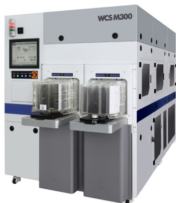
Figure 7. The WCS M300 automated VPD scanner system from NvisANA, Korea.
