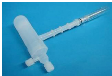
Figure 6. Inert (HF resistant), O-ring-free, PFA sample introduction system.
