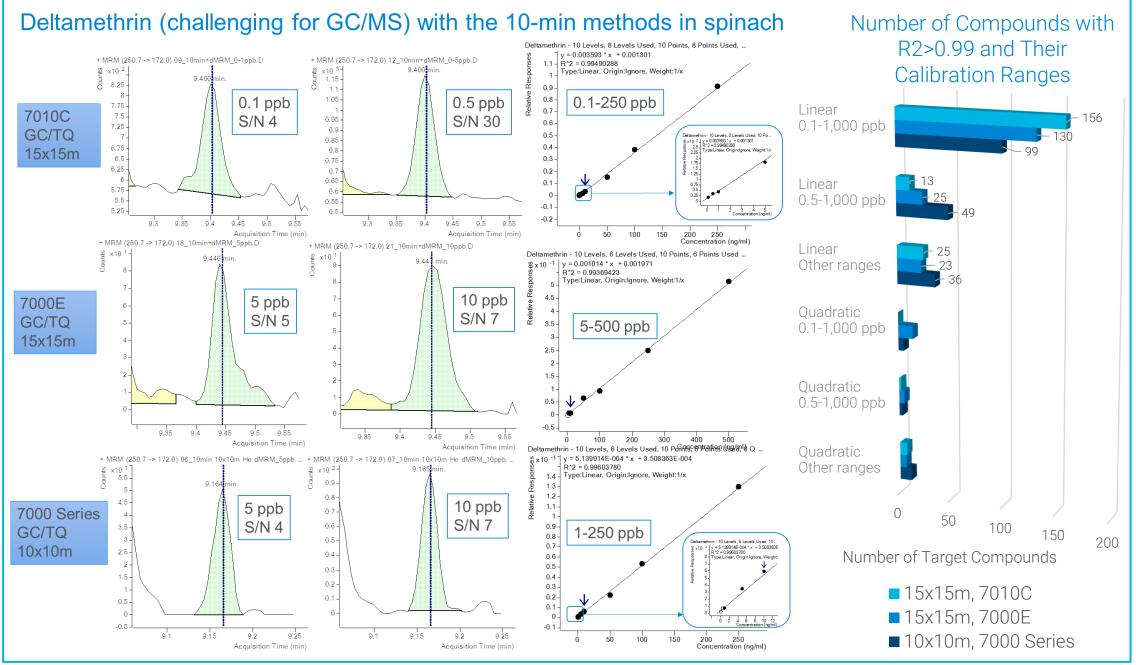
Figure 3. MRM chromatograms and matrix-matched calibration curves in spinach extract for deltamethrin (left) and the calibration performance for the 203 pesticides with the fast 10-minute methods in spinach (right).
