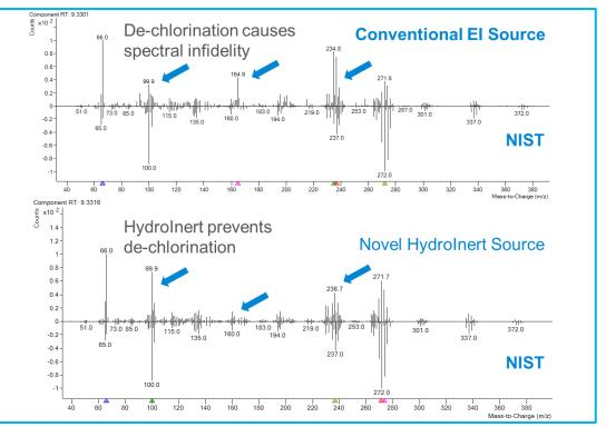
Figure 6. Mass spectra for heptachlor with hydrogen carrier gas
