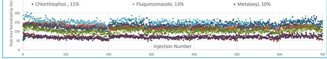
Figure 4. Stability of the peak area for pesticides spiked at 20 ppb into spinach extract normalized by the ISTD over 700 consecutive injections with the 10-min analysis using the conventional 15x15m column configuration.
