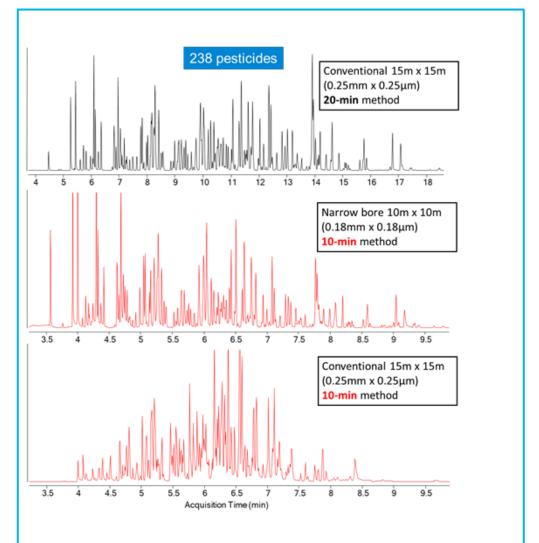
Figure 2. MRM total ion current chromatograms for a mixture of 238 pesticides acquired with the conventional 20-min method (top), fast 10-min method with the narrow bore configuration (middle), and fast 10-min method with the conventional 15x15m configuration (bottom).
