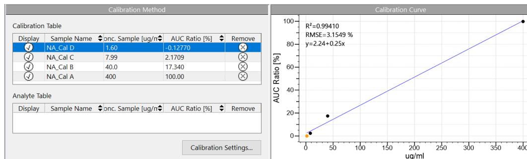
Statistics are reported in the calibration curve. The lower the **RMSE** (root mean squared error), the better the curve is fitting. The closer the  **$R^2$**  (coefficient of determination) is to 1, the better the curve is fitting.
