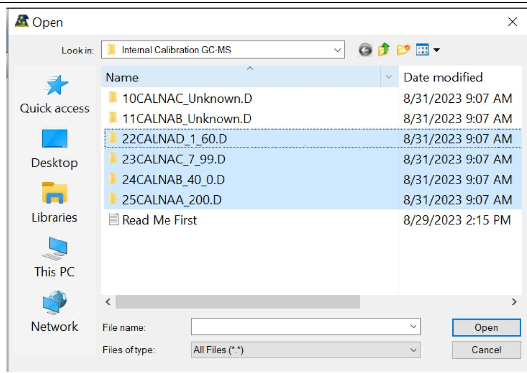
4 In the drop-down list, select the calibrant file where analyte concentration is the largest, in this example, it is the **25CALNAA\_200.D**
