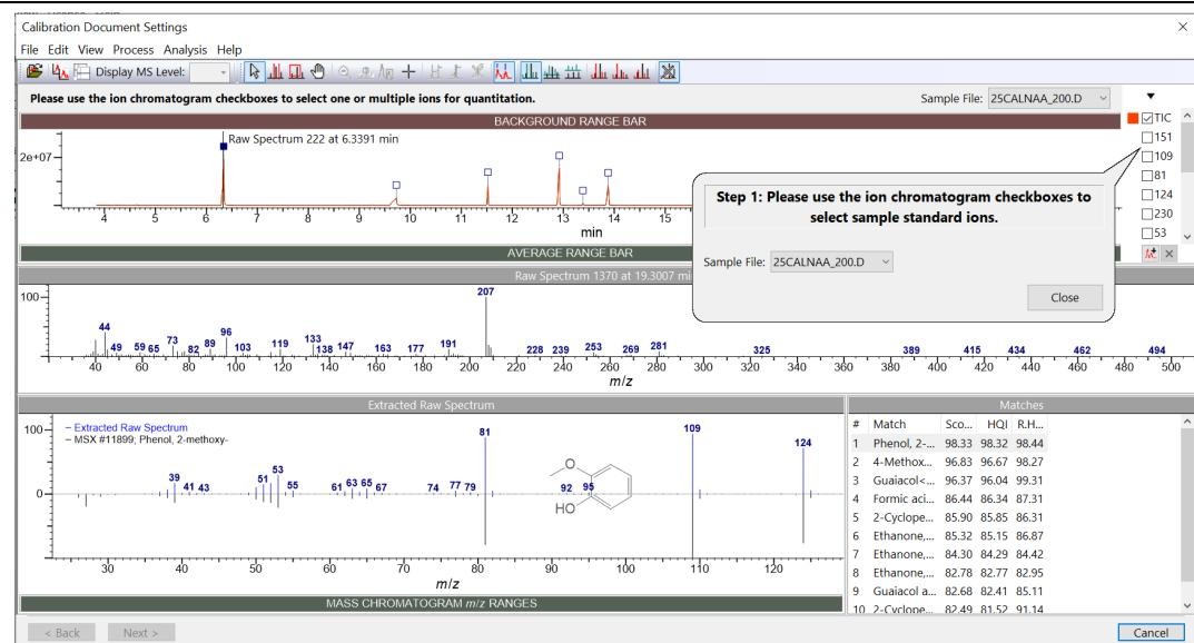
5 Select a component from the **Raw Spectrum** pane, in our example, the interested component has a TIC peak at **6.45** min.
