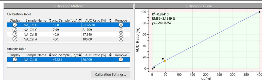
The concentration ratio of analyte to internal standard is shown in the **Analyte Table** and as a square spot in the **Calibration Curve**.
