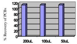
Amount of Methanol spiked into extraction vessel. Average % PCBs: 113%
