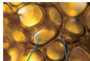
CO 2 filled cell cell wall Light Microscope Image of PU Foam
