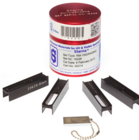
Figure 2. Metal-on-quartz filters used for the NIR photometric accuracy test of the Agilent Cary 7000 UMS. Photo reproduced with permission from Starna Scientific Ltd.
