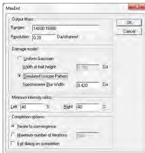
Figure 2.2.6. Typical parameters for MaxEnt processing the background-subtracted raw m/z data from 500-fold diluted blood samples. The Spectrometer Blur Width may need adjusting (0.3-0.5) to make the \alpha -chain mass within \pm 0.1 Da of its sequence mass.
