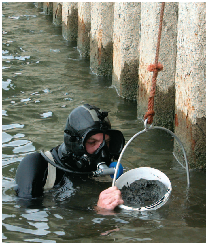
Figure 1: Obtaining of sediment samples from a harbor basin carried out by the German company Schreiber in Duisburg
