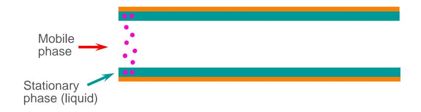
Solute molecules distribute into the two phases based on their degree of solubility/distribution in the stationary phase ( $K_c$ )
