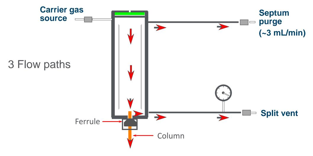
Flow through injector = Column flow + split vent flow
