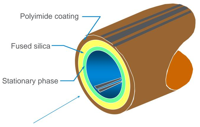
Expanded view of capillary tubing
