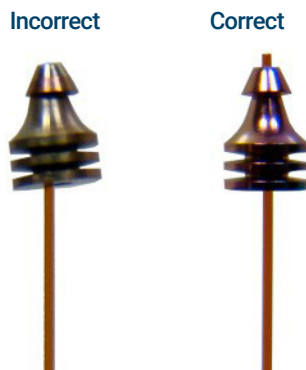
Figure 7. Incorrect and correct swaging symmetry.
