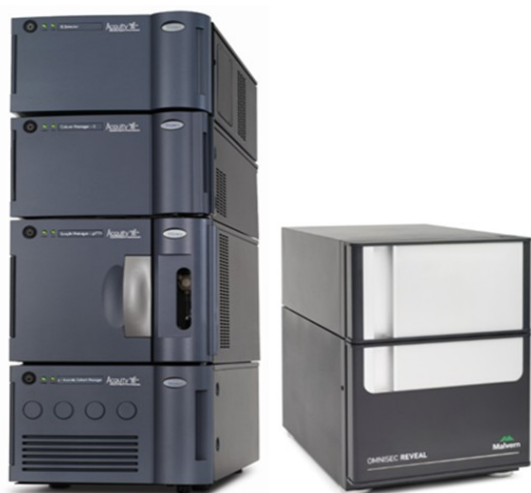
Figure 1. ACQUITY APC SEC Core 1 System with post column flow to the Malvern OMNISEC Reveal.
